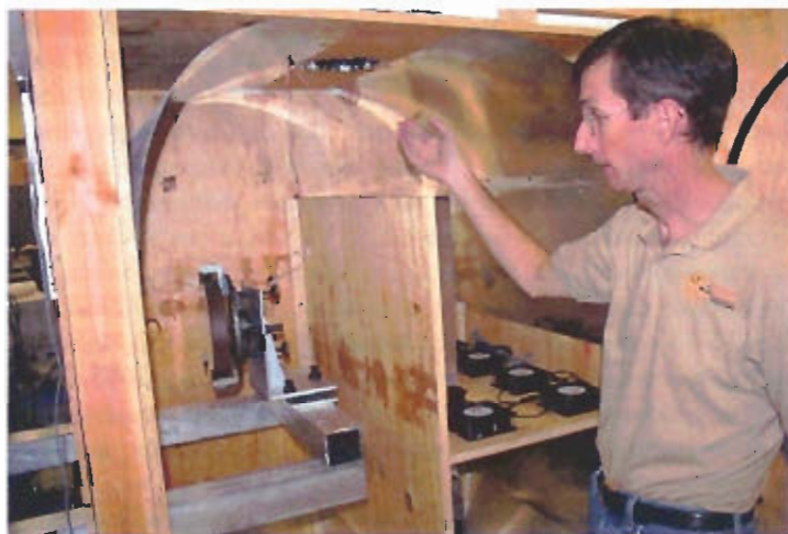
Rob Hubbard (Tucson) shows the interior of the air curtain experimental cabinet assembled at NOAO's Tucson optical shop. At left center is an optical flat to reflect light back into a Zygo interferometer after the light passes through a laminar air curtain formed by air exiting a bank of soda straws (below). The interior of the box simulates the warmer interior of the coudé rotator where M5 and M6 will be located. Preliminary on and off interferograms (bottom) show a marked improvement in internal seeing. (NSO/AURA/NSF)
