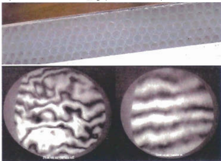
Rob Hubbard (Tucson) shows the interior of the air curtain experimental cabinet assembled at NOAO's Tucson optical shop. At left center is an optical flat to reflect light back into a Zygo interferometer after the light passes through a laminar air curtain formed by air exiting a bank of soda straws (below). The interior of the box simulates the warmer interior of the coudé rotator where M5 and M6 will be located. Preliminary on and off interferograms (bottom) show a marked improvement in internal seeing. (NSO/AURA/NSF)
